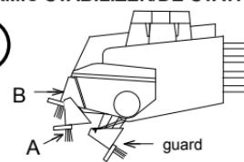
The M97xE's exclusive viscous-damped Dynamic Stabilizer ④ maintains a uniform distance between the cartridge and the record under difficult playing conditions, such as those caused by warped records or mismatched tonearm mass. When such stabilization is not required, the stabilizer can be locked into its up position, which can improve sound quality under ideal playing conditions.
